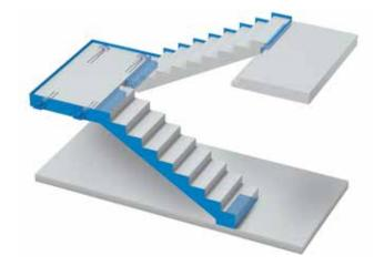
Straight staircase, landing decoupled. Schöck Tronsole® type P, F, B and L
